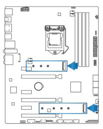
8. Insert the Sabrent ROCKET NVMe M.2 SSD device pin-side first into the M.2 slot as is illustrated below.
