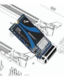
9. Fasten the opposite end of the **Sabrent ROCKET NVMe M.2 SSD** to the motherboard with the necessary screw or hardware, as is illustrated below.
